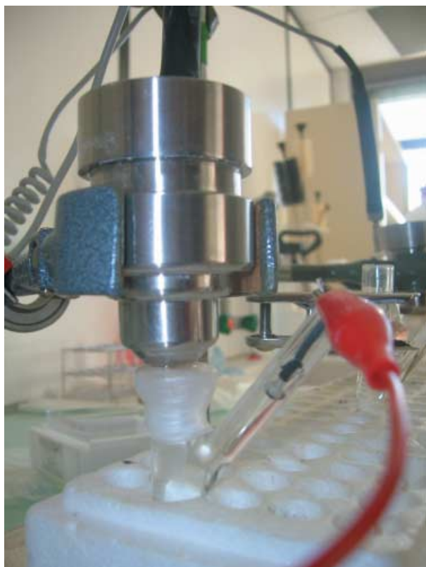
Figure 1 Experimental set-up for in vitro permeation studies. Gel 1-CAF and Gel 2-NAP (100 \mu L) were applied directly to the skin surface. Subsequently, the steel roll-on was placed in contact for the current application period with the device set at the appropriate polarity; the electrical circuit was completed by placing a return electrode in the sampling arm of the Franz cell, and in contact with the receiver phase.
